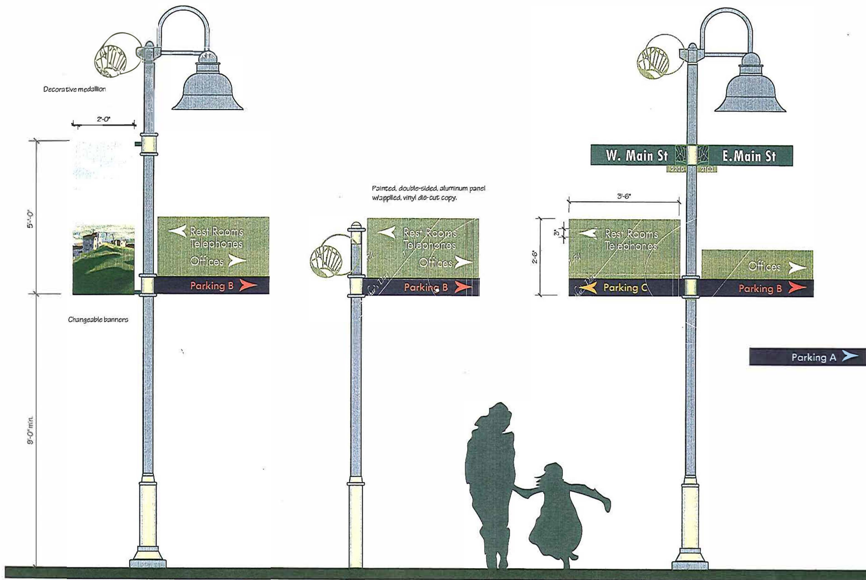
Elevation: Pedestrian Directional on light pole with banner scale: 1/2"=1'-0"
