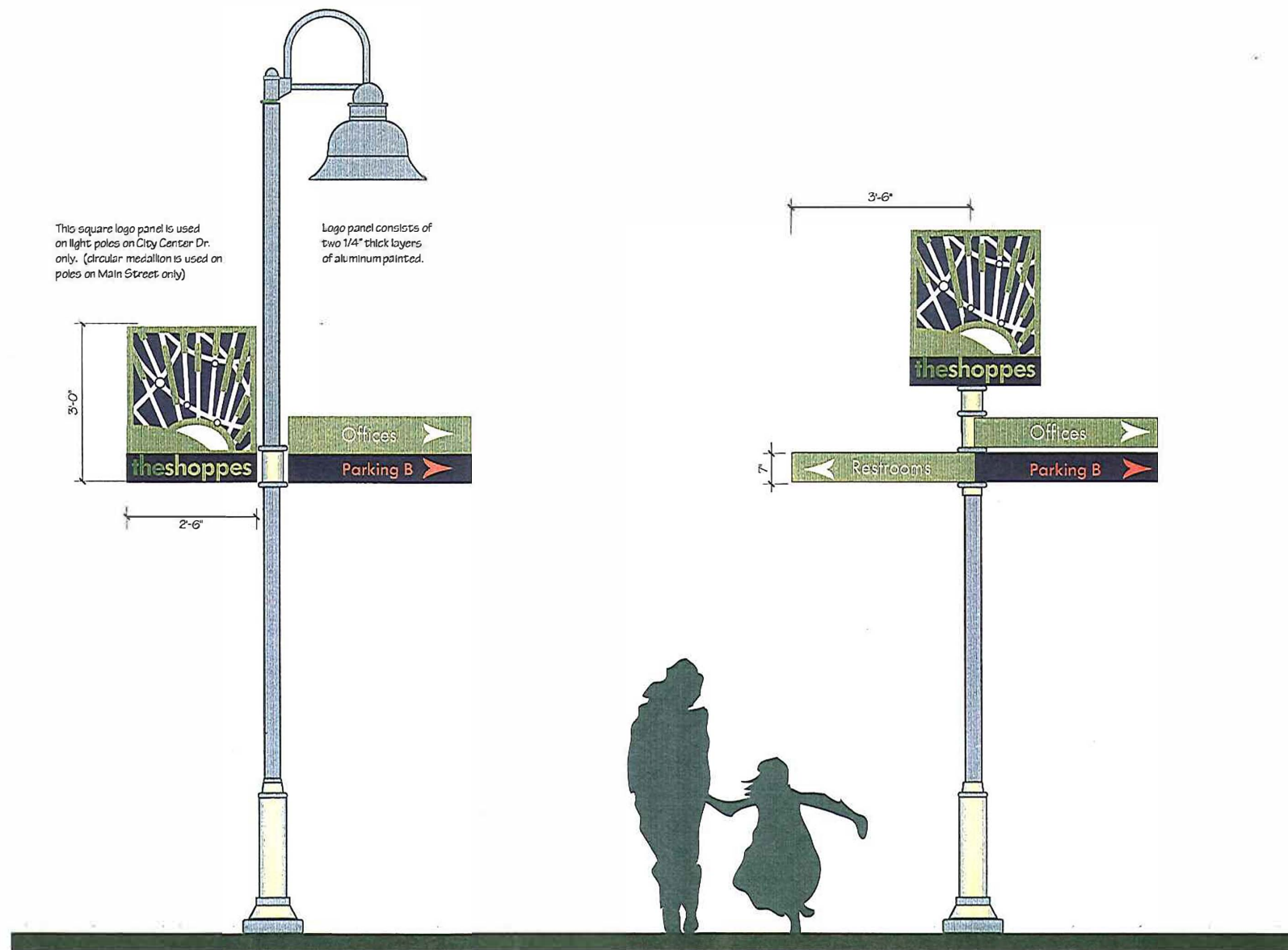
Elevation: Pedestrian Directional on light pole with logo panel scale: 1/2"=1'-0"
