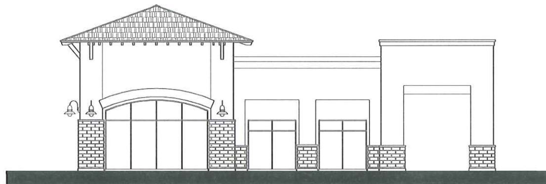
EAST ELEVATION - SHOP TENANT SCALE 1/16" = 1'-0"
