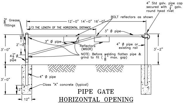
All joints welded in shop (No field welds).
